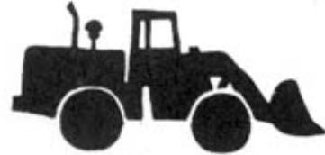
Articulated Loader (pivots in center)
